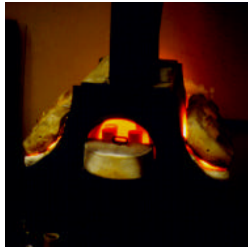
Muffle furnace isolated from the reducing conditions underneath
