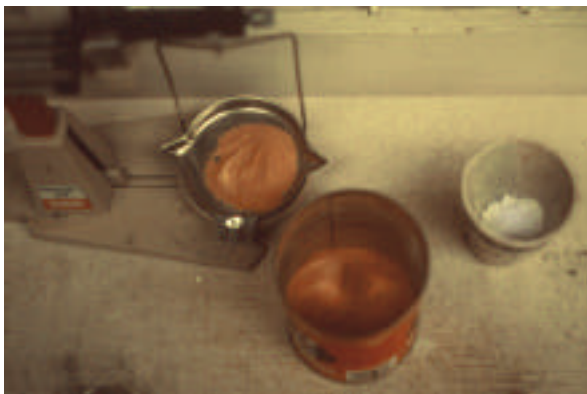
Litharge and soda being measured into a crucible
