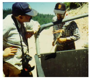
We pulled the vise-grip out of the tank after about a half an hour and found we had a lovely copper-plated tool for Charlie<sup>12</sup> to explain to his boss at the US Geological Survey. I took a small sample of the water from this tank, and let it congeal into crystals of green vitriol, which I then used to make a period leather dye. using a recipe from the 1548 Plictho of Gioanventura Rosetti. There is no vitriol left from this batch – I used all of it to make my leather dye.
